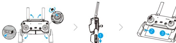
Unfold the antennas and mobile device clamps, then attach the control sticks.
